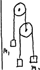
(The masses of the pulleys and friction are to be neglected)
